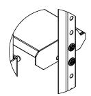
Mounts to existing storage posts at weight peg locations. Set to desired height and tighten with 1" mating bolts, tools provided. (For dumbbell setting, use second set of lower holes to place shelf at an angle.)
